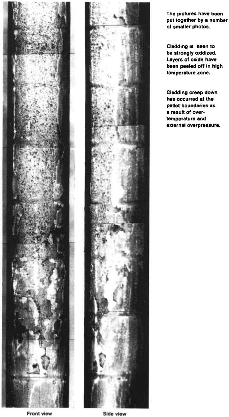
Figure 6. Hot cell pictures of the lower end of the dryout zone.
